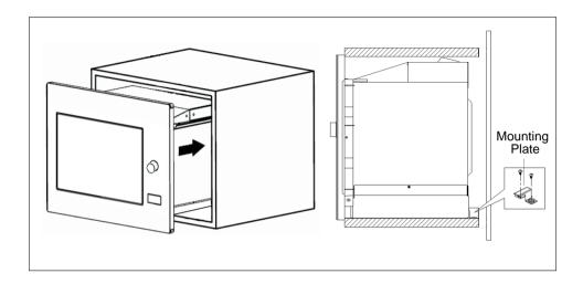
5. Open the door, fix the oven to the cabinet with screw at the installation hole. Then fix the Trim-kit plastic cover to the installation hole.
