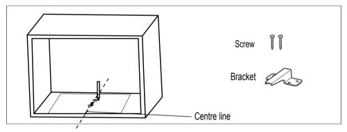
3. Remove the bottom cabinet template and fix the bracket with screw .
