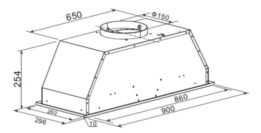
Create an opening in the underneath of the kitchen unit; the cut-out must be of the dimensions shown in the drawing below.
