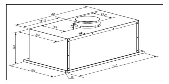
Create an opening in the underneath of the kitchen unit; the cut-out must be of the dimensions shown in the drawing below.
