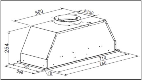
Create an opening in the underneath of the kitchen unit; the cut-out must be of the dimensions shown in the drawing below.
