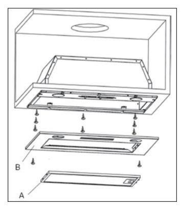
3) Make a hole in the inside of the kitchen unit for the electrical cable to feed through. Remove the 2 screws securing the extractor frame (B) to the hood and unscrew the 2 lights. Ensure that the two support clips on either side of the hood are set to accommodate the thickness of the mounting surface, by adjusting the clip via the screw.
