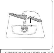
To remove the lower spray arm, pull out the spray arm upward.
