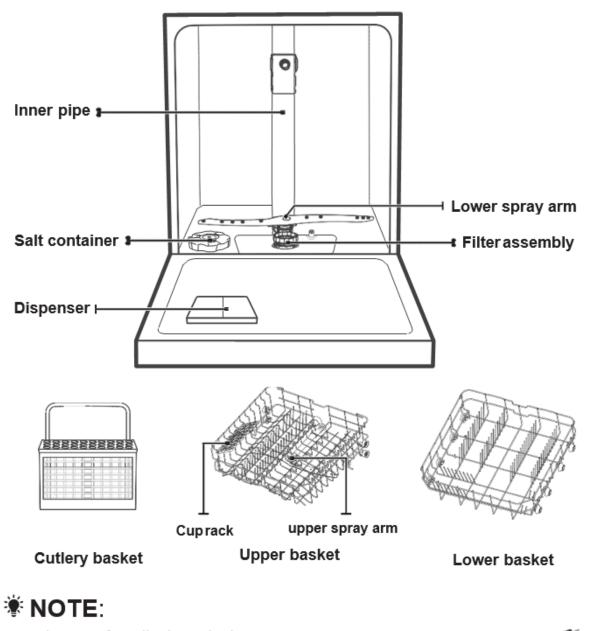
To make room for taller items in the upper basket, raise the cup rack upwards. You can then lean the tall glasses against it. You can also remove it when it is not required for use.
