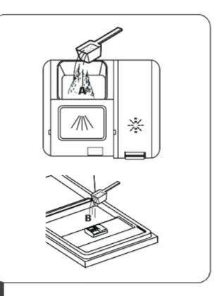
Add detergent into the larger cavity (A) for the main wash cycle . For better cleaning result, especially if you have very dirt items, pour asmall amount of detergent onto the door. The additional detergent will activate during the pre-wash phase.
