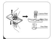
The fine filter can be pulled off the bottom of the filter assembly. The coarse filter can be detached from the main filter by gently squeezing the tabs at the top and pulling it away.
