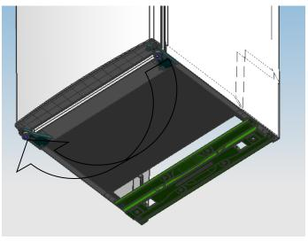
6) Set the door right position ,fix the mid-hinge .
