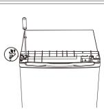
8. Put the top cover and fix it with 2 screws on the back.
