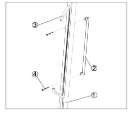
screw-driver (4) Put back door seal to cover the screws.
