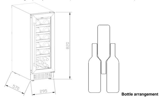
Loading capacity will vary in terms of different way of bottle arrangement or different bottle sizes.
