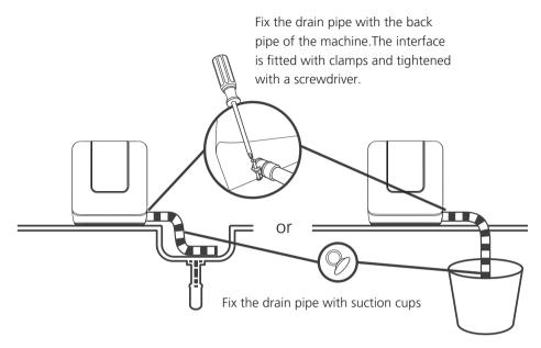
The connection of the drain pipe: Put end of the drain into a sink or bucket.
