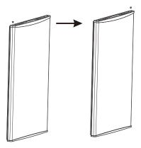
5)Install the door on the lower hinge assembly, and then install the upper hinge, hinge cover, pins and hole cap in sequence.
