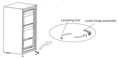
4)Dismantle the hole cap under the door, then assemble the hole cap on the other side.
