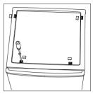
Unscrew top hinge and then remove upper door and place it on a soft pad to avoid scratch.
