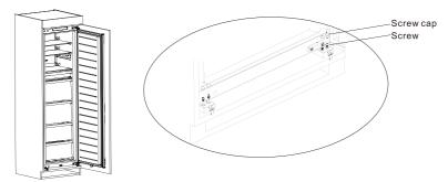
• Fix the top baffle to the top of the cabinet inner with screws, then install the screw caps.
