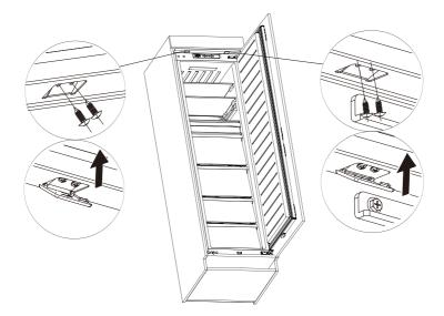
• Open the door of cabinet the maximum angle, and open the door of the refrigerator to the corresponding position. Sliding the block to make sure inner edge align with the door edge of refrigerator, then fix the block to the door of cabinet with screw and install screw caps.
