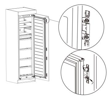
• Take out the sealing strip from accessory bag, and press it in the gap between the cabinet and the refrigerator. Installation is completed.
