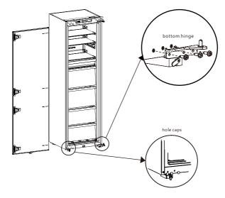
4) Exchange the bottom hinge and upper hinge  $% \left( {{\rm D}} \right)$  , then install them according to below steps, and install the top hole caps.
