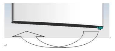
6) Replace the bottom hinge to the other side then fix it with screws.
