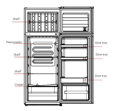
Drawers, food boxes, shelves, etc. placed according to the position in the picture above are the most energy efficient.
