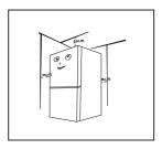
• The top space of the refrigerator shall be greater than 30cm, and The refrigerator should be placed against a wall with a free distance more than 10cm to facilitate heat dissipation.
