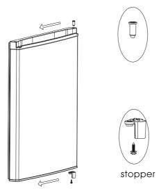
6)Put the freezer door on bottom hinge, then install the middle hinge and screw hole caps (a). Dismantle the door stopper of refrigerator door, and install it on other side by fitting screw (b).
