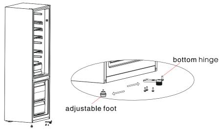
5) Dismantle the door stopper of freezer door, and install it on other side by fitting screw.
