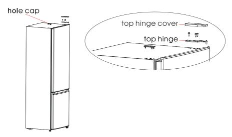
3)Remove the refrigerator door, middle hinge, and screw hole caps of the other side.
