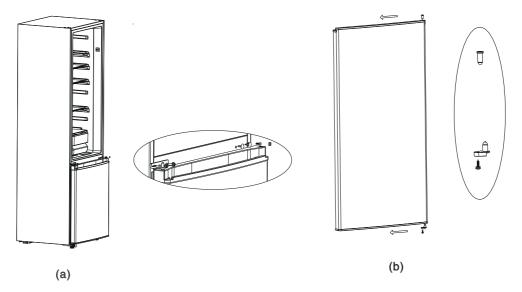
7) Change the installation position of top hinge shaft as shown as below, then put the refrigerator door on middle hinge, and fix the top hinge by fitting screws, finally to install the top hinge cover and hole cap.
