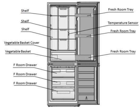
Drawers, food boxes, shelves, etc. placed according to the position in the picture above are the most energy efficient.
