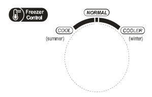
The freezing temperature is relatively low in "COOLER" position, while the freezing temperature is relatively high in "COOL" position, thus, "NORMAL" position is generally used.
