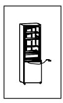
14) Assemble door shaft sleeve and door holder of freezing chamber to the other side of the door
