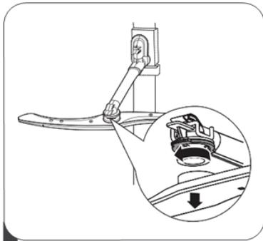
**1** To remove the upper spray arm, hold the nut, rotate the arm clockwise to remove it.
