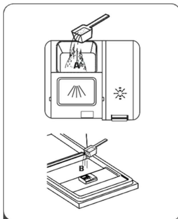
**2** Add detergent into the larger cavity (A) for the main wash cycle .
