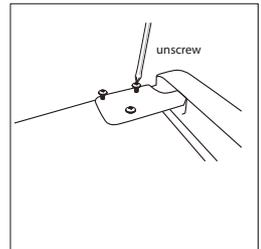
3. Remove the pin with a screwdriver and flip the hinge bracket. Then refit the pin to hinge bracket.
