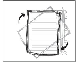
10. Make the middle hinge reverse the direction 180°C, then transfer it to the left property position. Make the middle hinge pin in the upper hole of the lower door, then tight the bolts.
