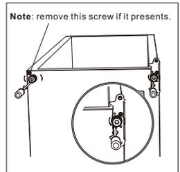
7. Unscrew and remove the bottom hinge pin, turn the bracket over and replace it.
