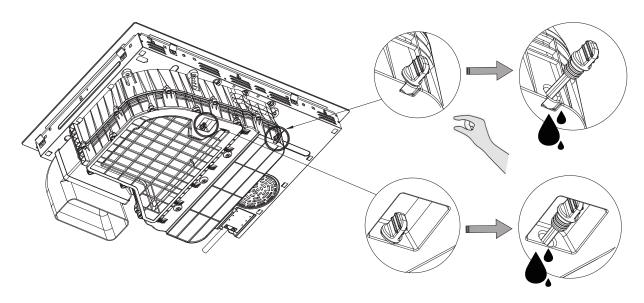
After draining water or installing the equipment, press the rubber plug tightly
