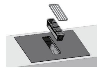
3. Remove the two odour filters, and dispose of them properly.
