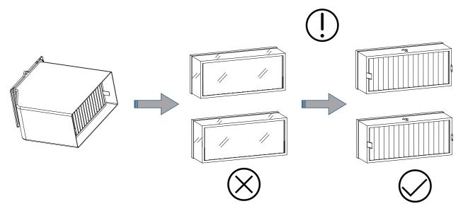
Before using the deodorizing filter element, tear off the outer transparent film.
