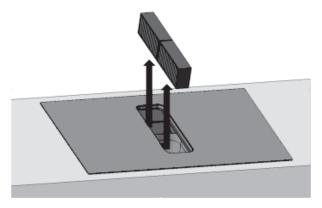
4. Insert two odour filters into the left of the appliance.
